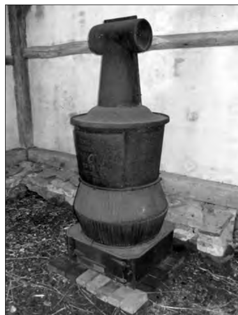
Oriskany Falls hop stove with a cast-iron T-joint stovepipe support.
